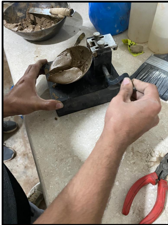
Figure 4.4: Casagrande cup experiment for Liquid limit test.
