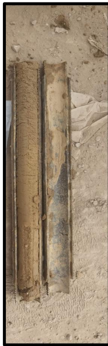
Figure 4.2: Equipment used in SPT Test. (1. Straight Rotatory drilling machine, 2. Split Spoon sampler, 3. Sample from the borehole).
