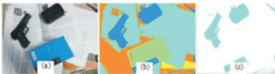
Figure 2.2: (a) Referenced image; (b) Segmented image; (c) Extracted gun color part from referenced image [10]
