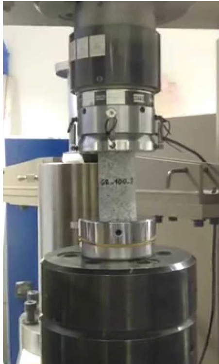
Figure 4.1. Uniaxial compression test machine
