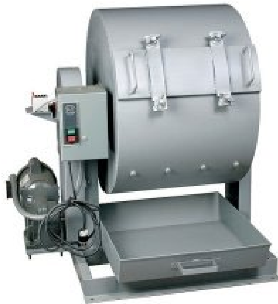
Figure 4.2. Machine of Los Angeles abrasion test
