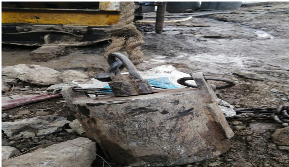
Figure 3.3 Drop hammer of 63.5kg used for SPT.
