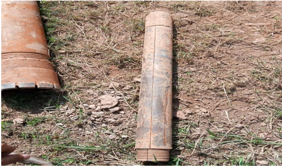
Figure 3.2 Split Spoon Sampler
