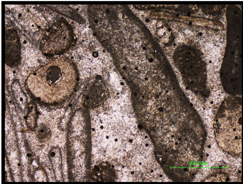
Plate 6.5. Petrographic interpretation shows micritic envelop around bioclasts and micritize bioclasts.
