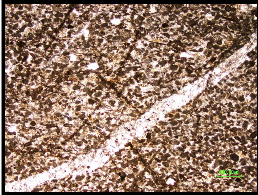
Plate 6.4. Petrographic interpretation exhibit calcite filled fracture along micritic peloids.
