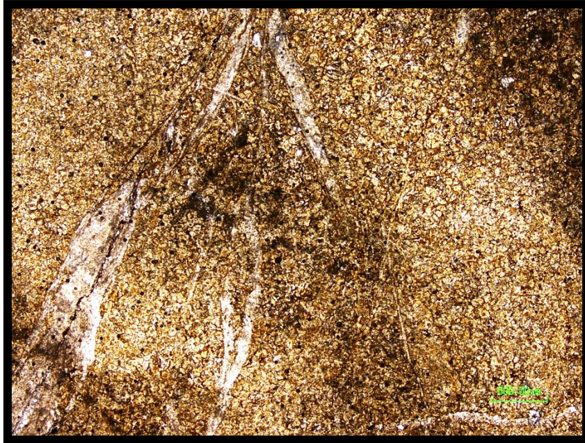
Plate 6.6. Petrographic interpretation of samples SKTS-6, SKTS-8, SKTS-11, SKTS-12, SKTS-16 shows pervasive dolomitization.
