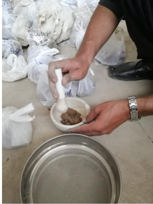
Figure.4.6. Using pestle and mortar to crush the lumped soil.
