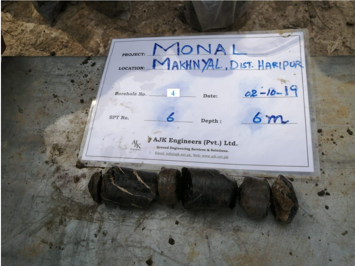
Figure 4.2. Samples taken out from SPT test at BH-4 depth 6m.
