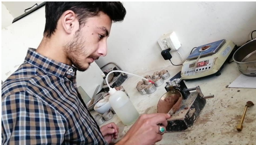
Figure 4.25. Carrying out the liquid limit test by Casagrande's method.
