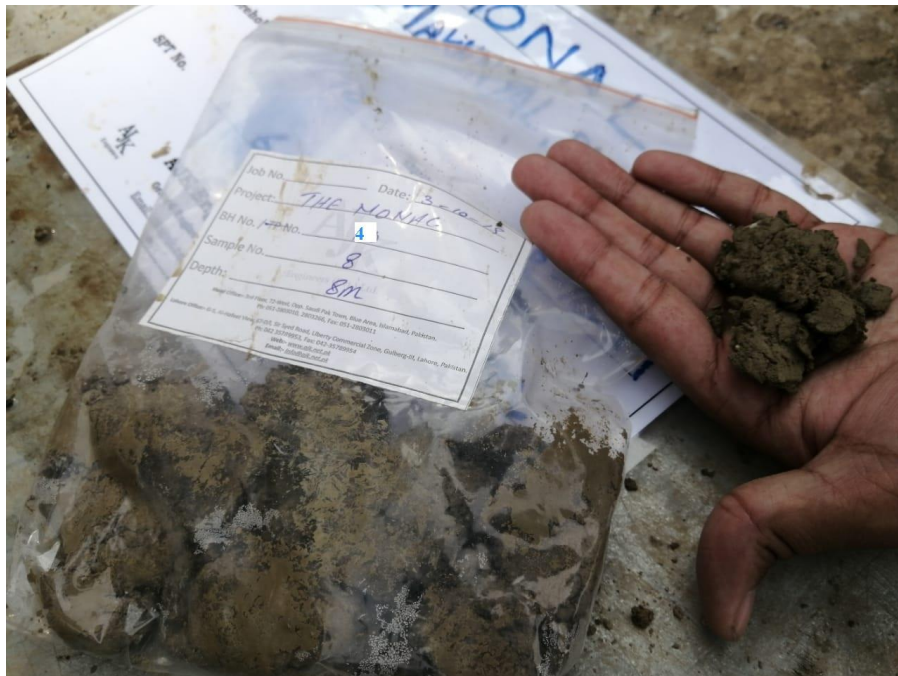
Figure 4.3. Samples from BH-4 being put in the polythene bag to maintain moisture.
