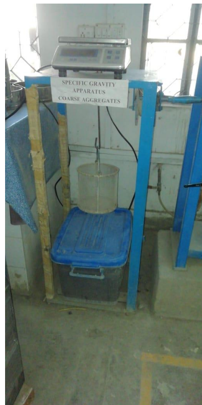
Figure 4.2. Specific gravity test being performed on the Malakand granite sample
