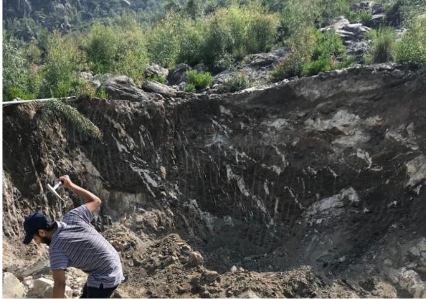
Figure 1.5. Weathered color of the Malakand granite.
