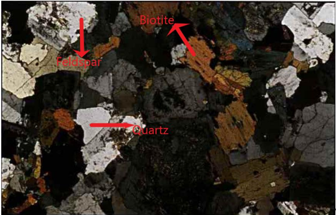
Figure 5.3. Quartz, feldspar and Bitotite grains shown in cross polarized light with 10X magnification.
