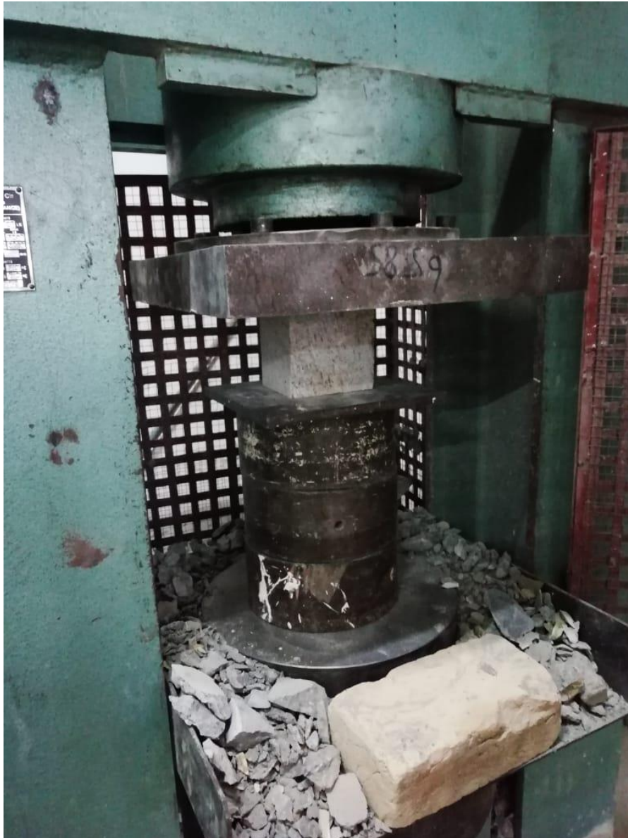
Figure 4.1. shows that the compressive strength test being performed on the cube sample of granite.
