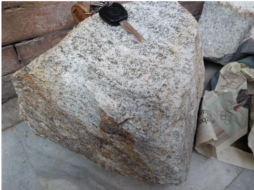
Figure 1.6. Fresh color of the Malakand granite sample.
