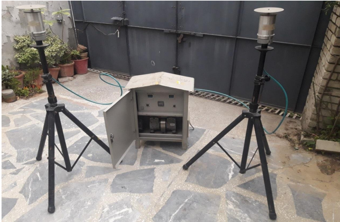
Figure 2.7 Low volume dual air sampler for particulate matter sampling
