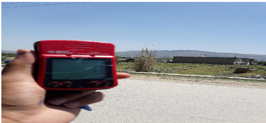
Figure 2.6 Smart sensor AS8700a for carbon monoxide sampling
