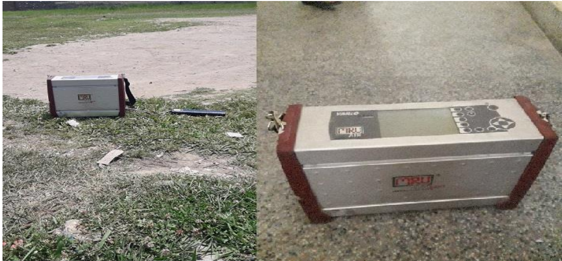
Figure 2.5 Vairo plus MRU for SO 2 , NO 2 and O 3 sampling
