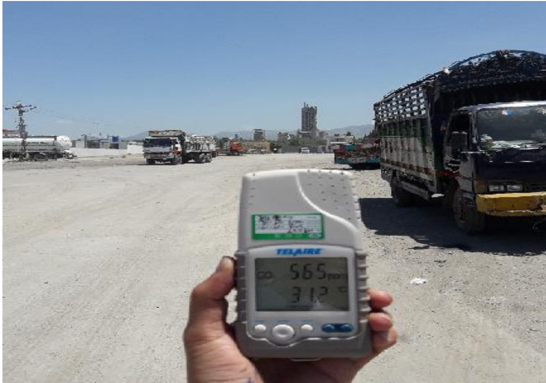
Figure 2.4 Telaire 7001 for carbon dioxide sampling
