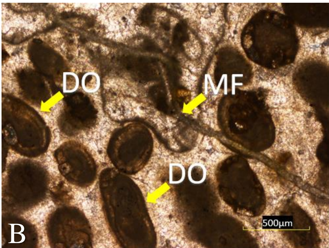
Plate 4.2.1.1.6 Photomicrograph (A) displaying Deformed ooids of concentric type (DO) with lamina of 5-10µm along with a calcite vein (CV) cutting across the thin section. Photomicrograph (B) displaying Deformed ooids of concentric type (DO) with lamina of 10-15µm along with a microfracture (MF) cutting across the thin section.
