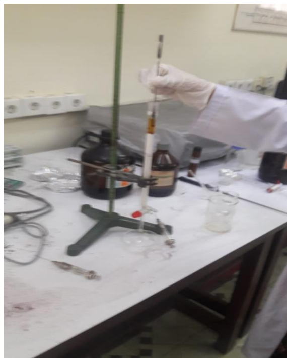
Figure 3.7. Aromatic fractions (pale color) of maltenes being eluted by DCM.
