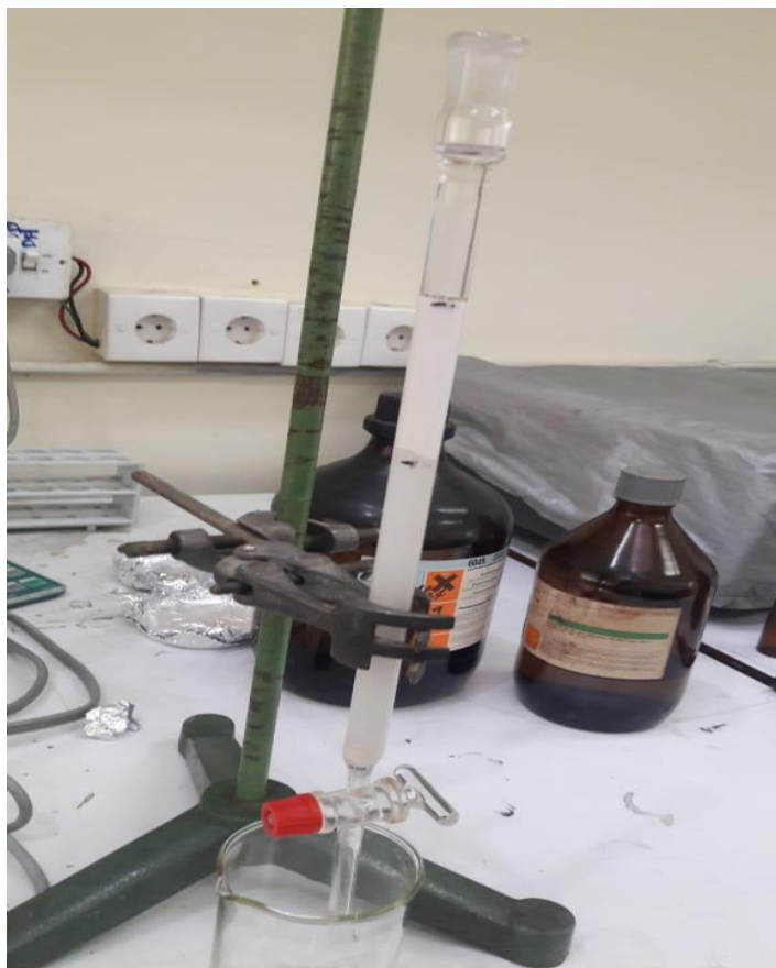
Figure 3.6. Glass column packed with silica and alumina for the separation of maltene fractions
