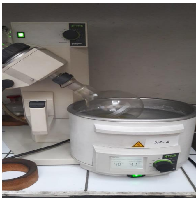
Figure 3.5. Evaporation of excess of organic solvent rotavapor.
