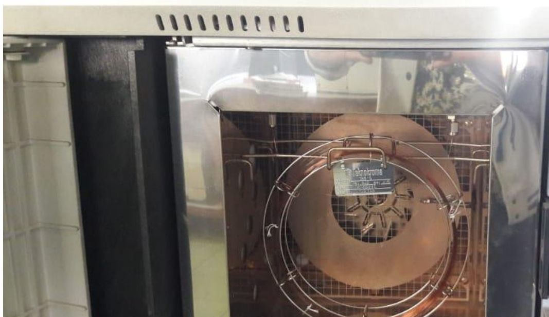
Figure 3.9. Auto XL Gas chromatograph at the top used to study seeps and GC oven housing column in bottom figure.
