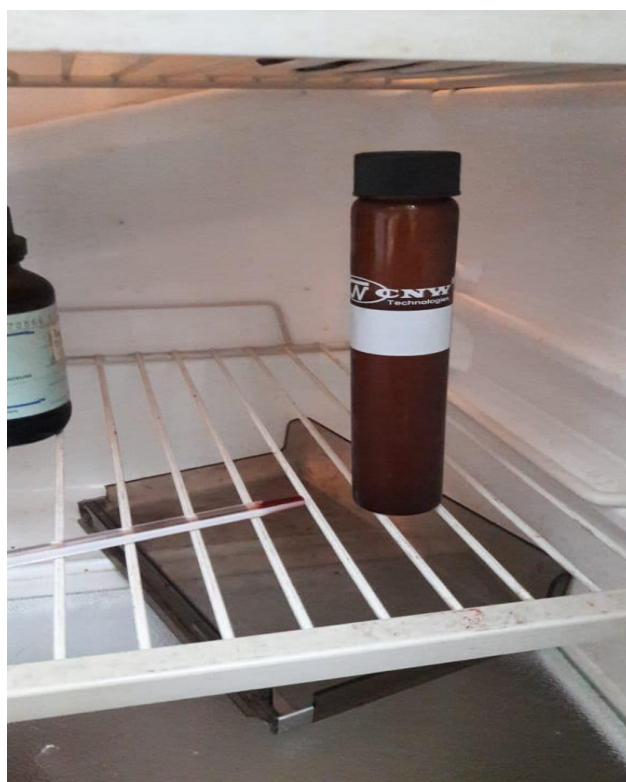
Figure 3.3. Addition of n-pentane and refrigeration of samples for precipitation.
