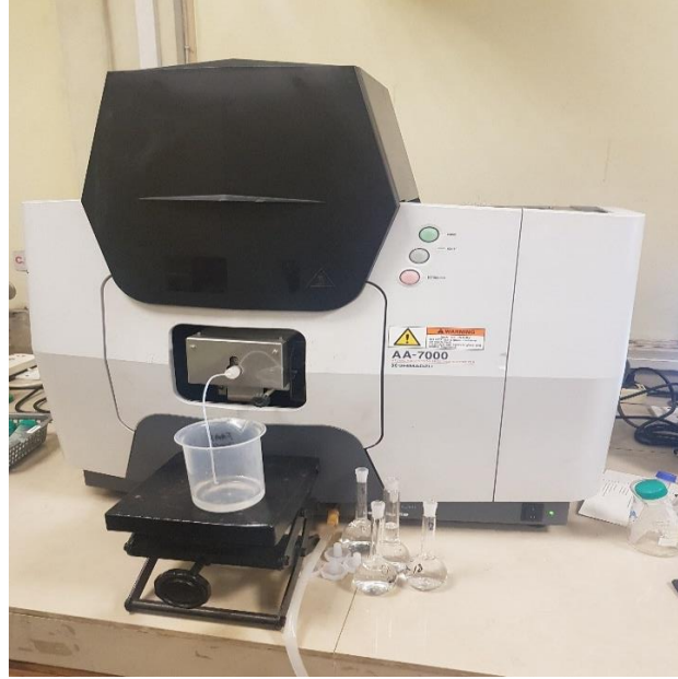
Fig 2.3: Instrument used to detect heavy metals in waste water samples.
