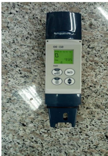
Fig 2.2: pH meter to determine pH, TDS, conductivity and salinity.
