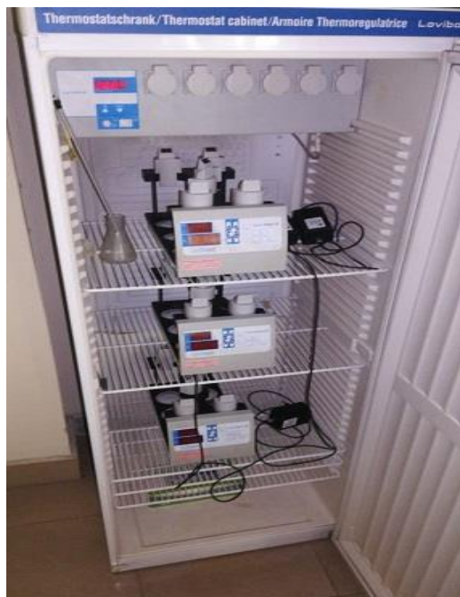
Fig 2.5: Thermostat cabinet used for the measurement of BOD.
