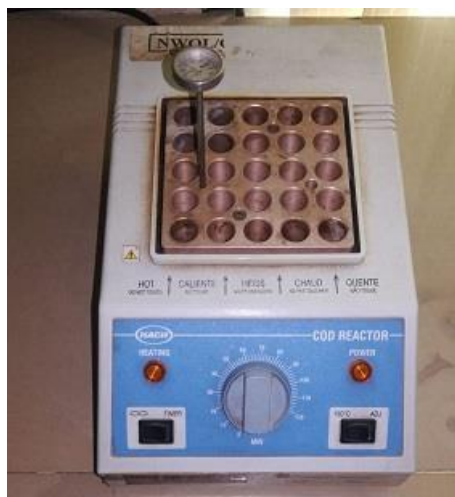
Fig 2.4: Equipment used for the measurement of COD in waste water samples.
