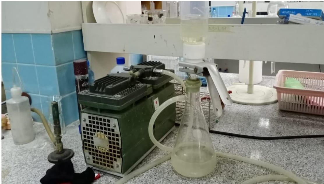
Figure 7. TSS filtration chamber and suction pump
