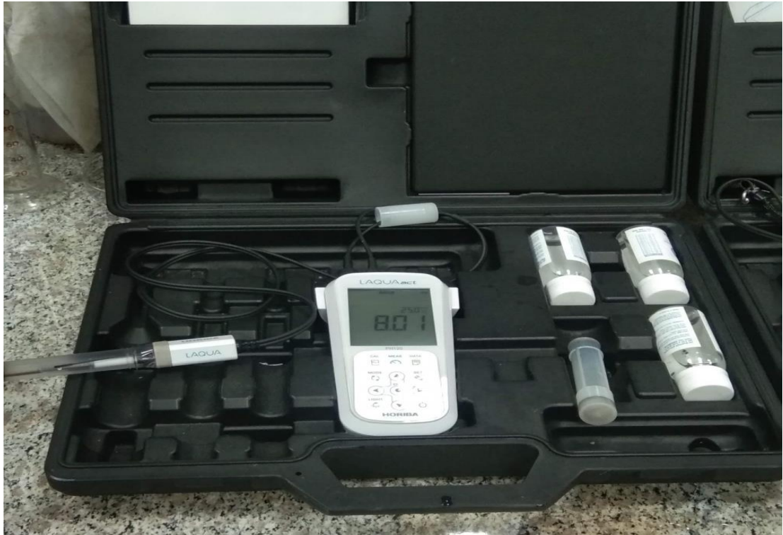
Figure 5. On-site mobile pH meter
