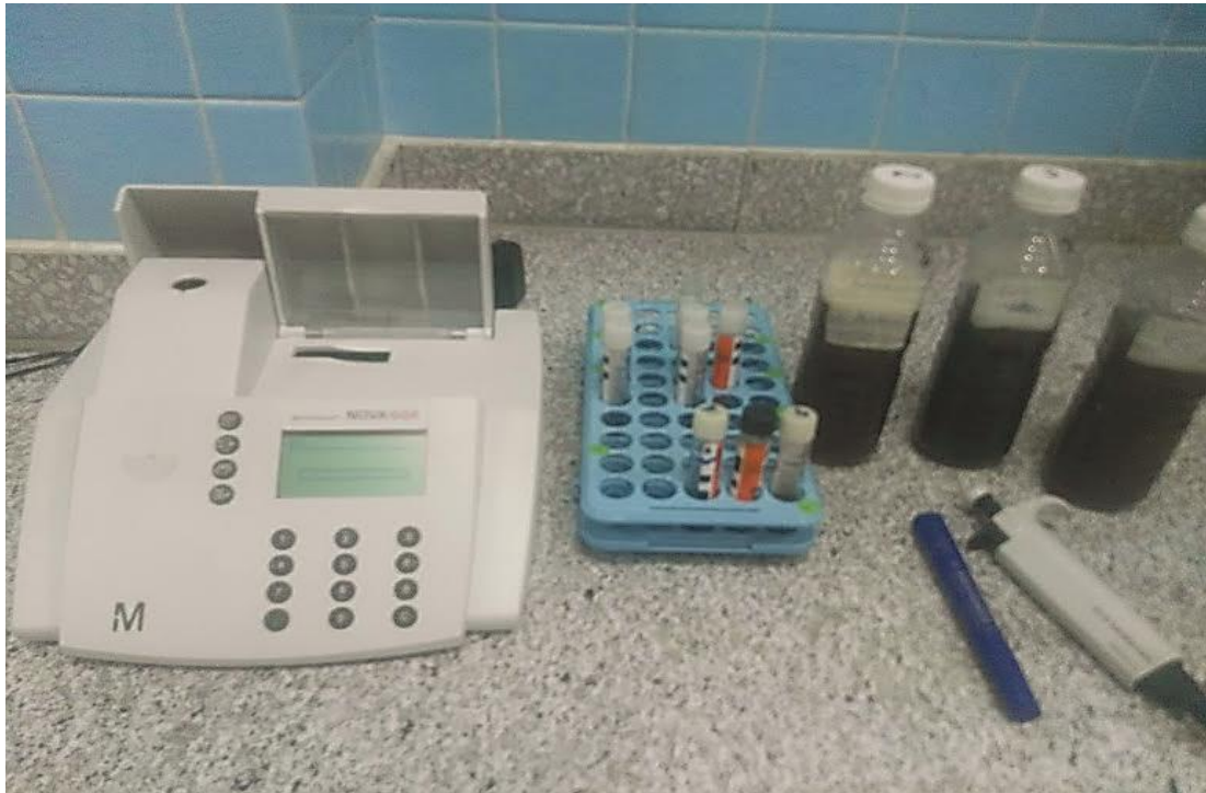
Figure 10. Test tube method for Heavy metal testing at NOVA 60.
