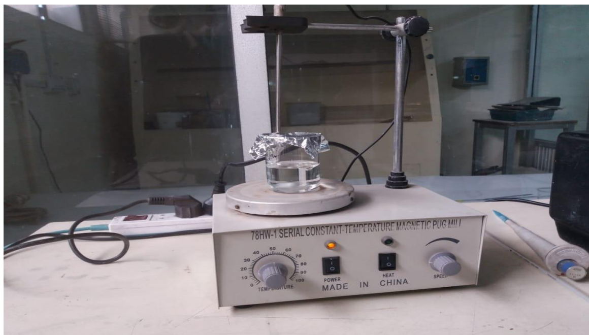
Figure 3.5 Toluene heating process and mixture of polyethylene.
