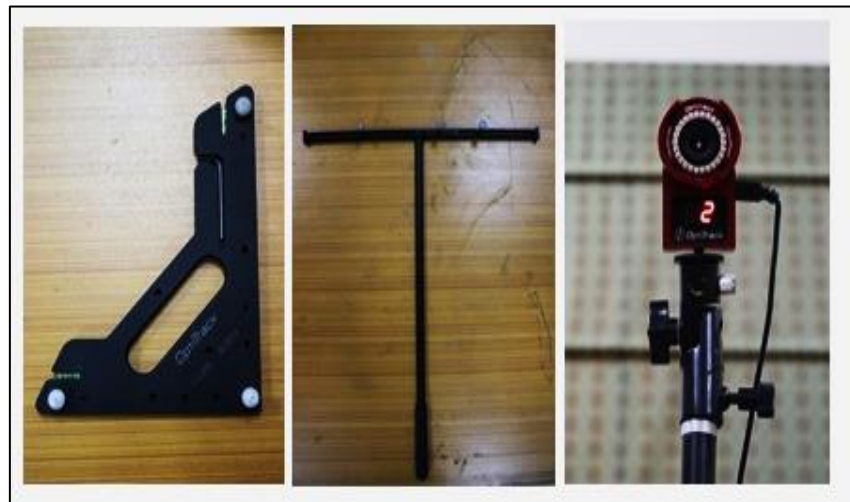
Figure 4.3. From left to right; calibration square, calibration wand, infrared camera by OptiTrack
