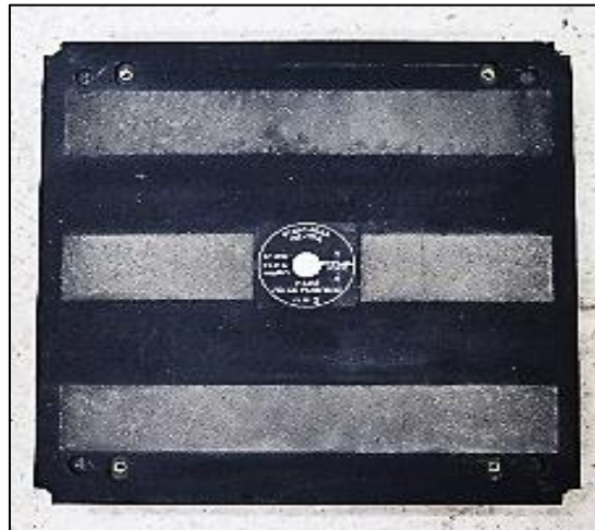
Figure 4.4. Force data were captured by 2-axis 4-beam Pasco force platform
