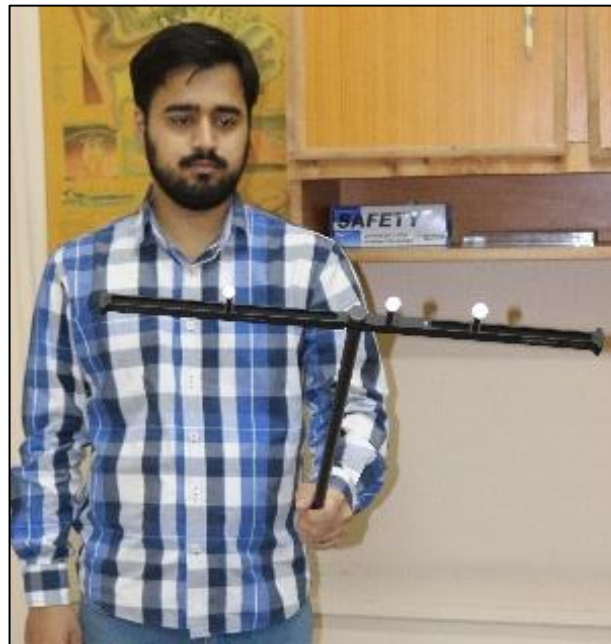
Figure C. 3. A calibration wand is used to tune camera measurements
