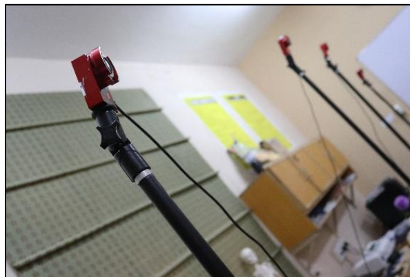
Figure C. 1. Four Flex 3 cameras set up to capture STS motion
