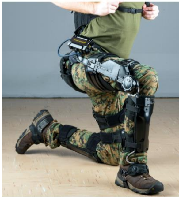
Figure H. 1. Knee exoskeleton for force augmentation of soldiers
