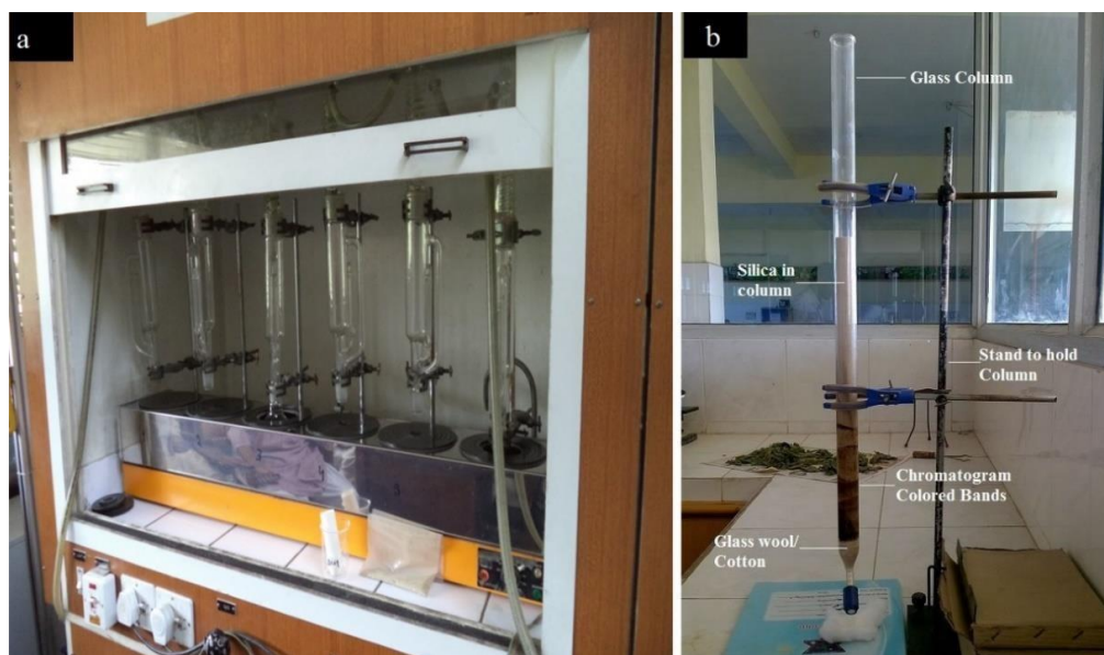
Figure 3.6 Fractionation of different chemical compounds, a) Soxhlet and b) Column Chromatography.
