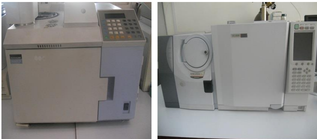
Figure 3.8 Gas Chromatograph mass spectrometer(GC-MS).
