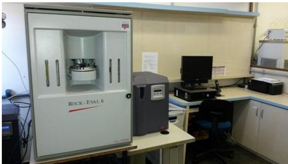
Figure 3.3 Showing Rock Eval-6 used for pyrolysis.
