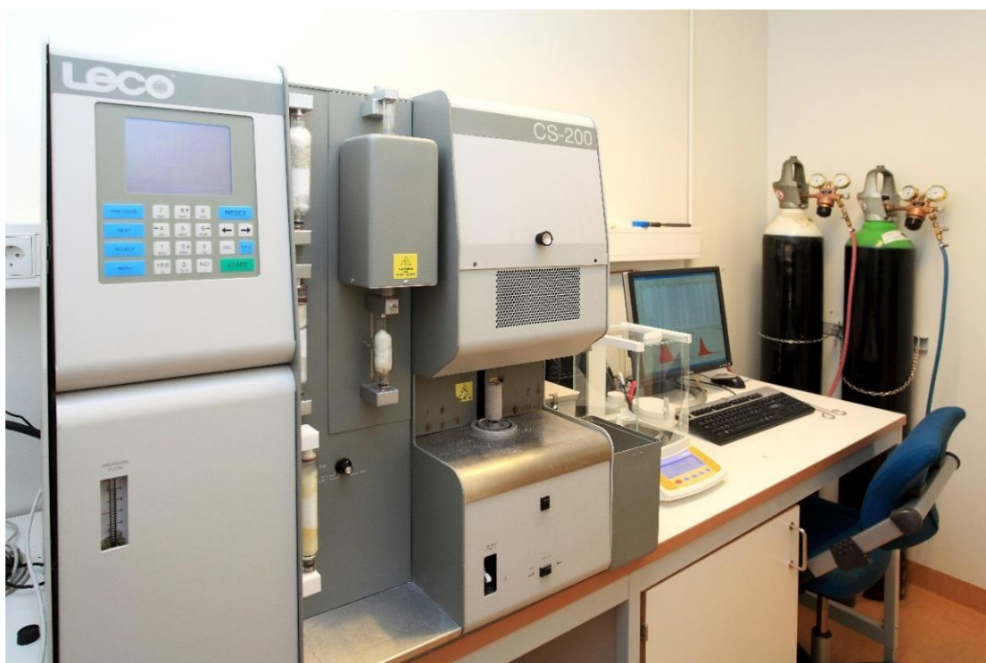
Figure 3.1 Equipment used for TOC determination (LECO CS-300).
