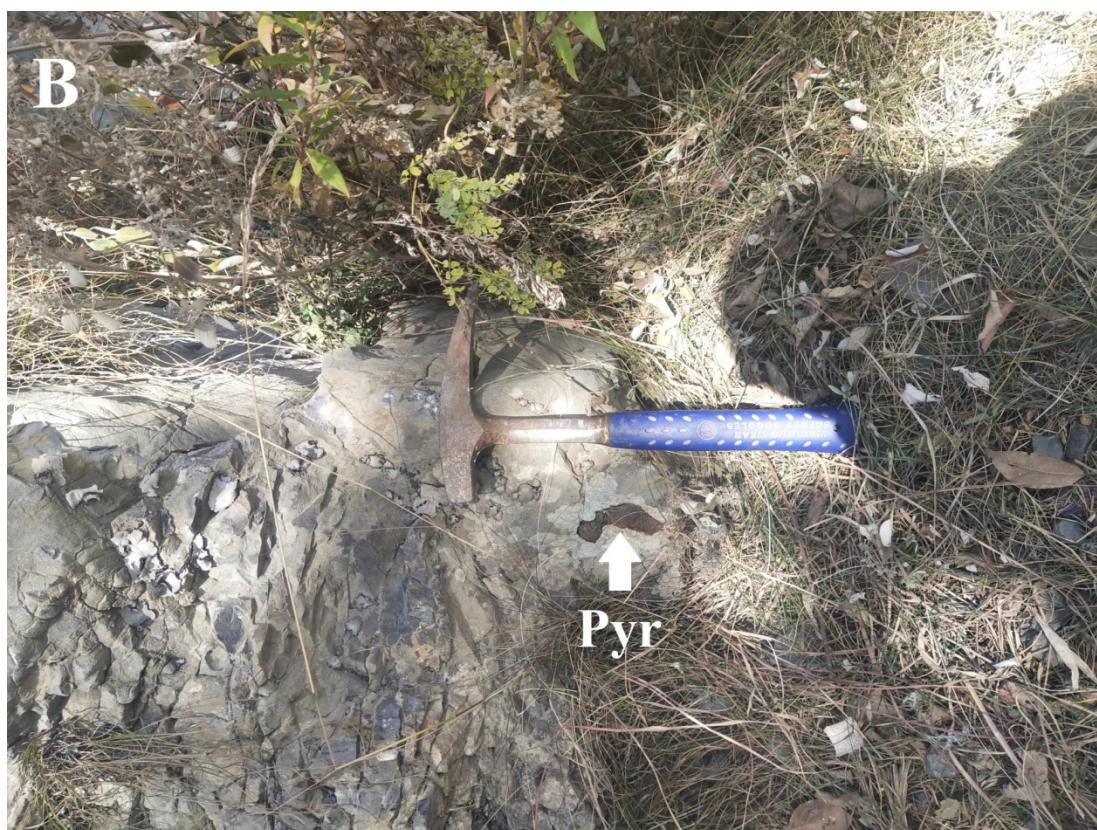
Figure 1.4 Field photographs of the Kawagarh Formation, A) showing iron leaching indicated by brown patches and B) showing pyritization (Pyr).
