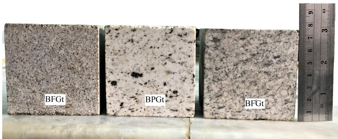
Figure 4.1: Cube samples of the different rock textural varieties from the Bibior area. BFGt; Bibior Fine-grained Granite, BPGt; Bibior Porphyritic Granite, and BF'Gt; Bibior Foliated Granite.
