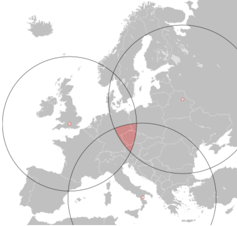
Figure 2.2: Example of Nearest Neighbors using monitors in the UK, Italy, and Belarus. The red area represents the range of Target [20]
