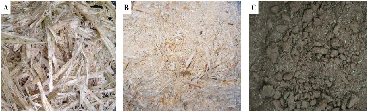
Figure 2.2 (A) Raw Sugarcane Bagasse (SB), (B) SB Powder (C) SB after pyrolysis
