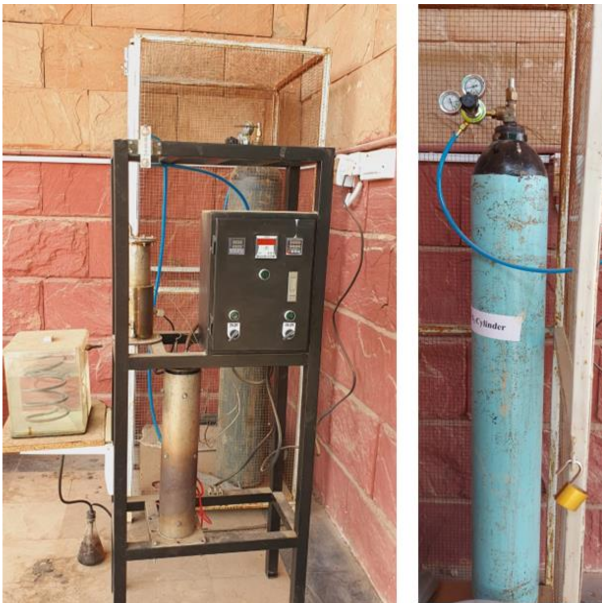
Figure 2.4 (A) Bench Scale Fixed Bed Reactor, (B) N 2 cylinder
