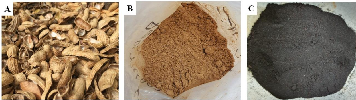
Figure 2.3 (A) Raw Peanut shell (PS), (B) PS Powder (C) PsS after pyrolysis
