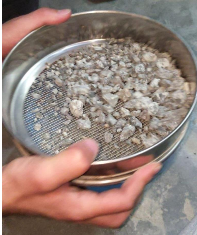
Figure 3.4. Sieving of the load applied aggregate.
