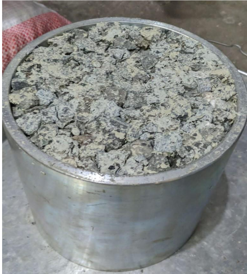
Figure 3.3. Aggregate in cylinder after apply load in machine
