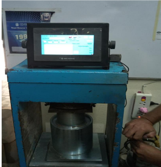
Figure 3.5. Aggregate crushing test machine
