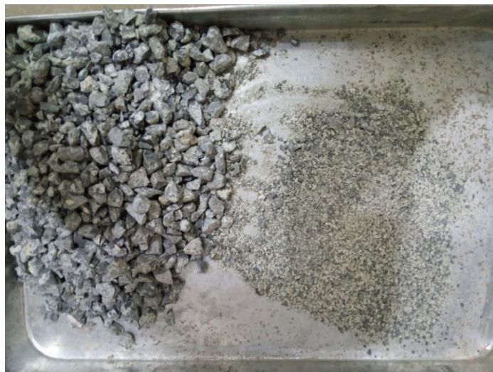
Figure 3.6. Crushed aggregate after sieving
