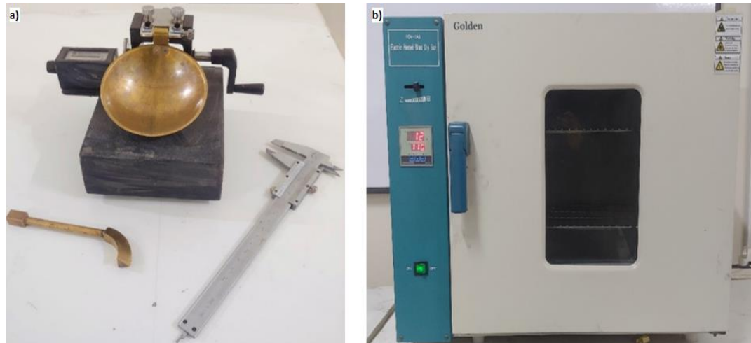
Figure 3.1 a) Casagrande apparatus for the liquid limit test, b) oven for drying samples.
