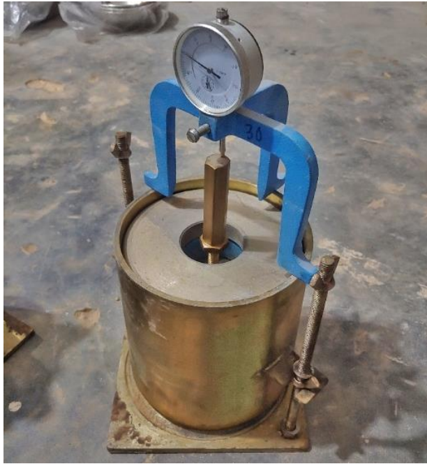
Figure 3.6 CBR sample in mold ready to soak.
