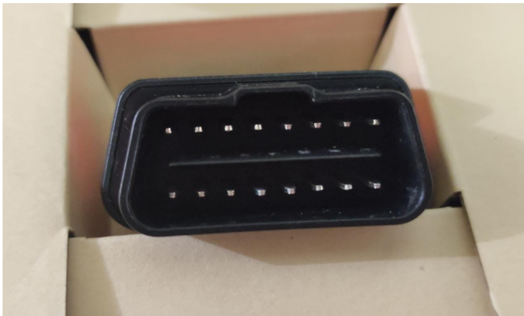
Figure 2.27: Ancel OBD-II Scanner (Back)
