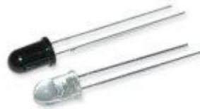
Figure 13: Infrared transmitter (BELOW) and infrared receiver (ABOVE). [Ref 4]
