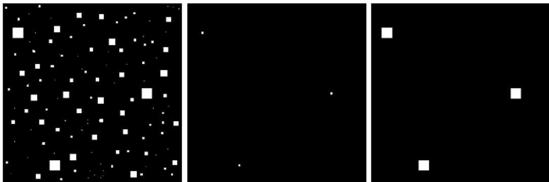
Figure 23: Opening operation. Original Image (LEFT). Eroded Image (Centre). Dilated Image (Right). [Ref 2]
