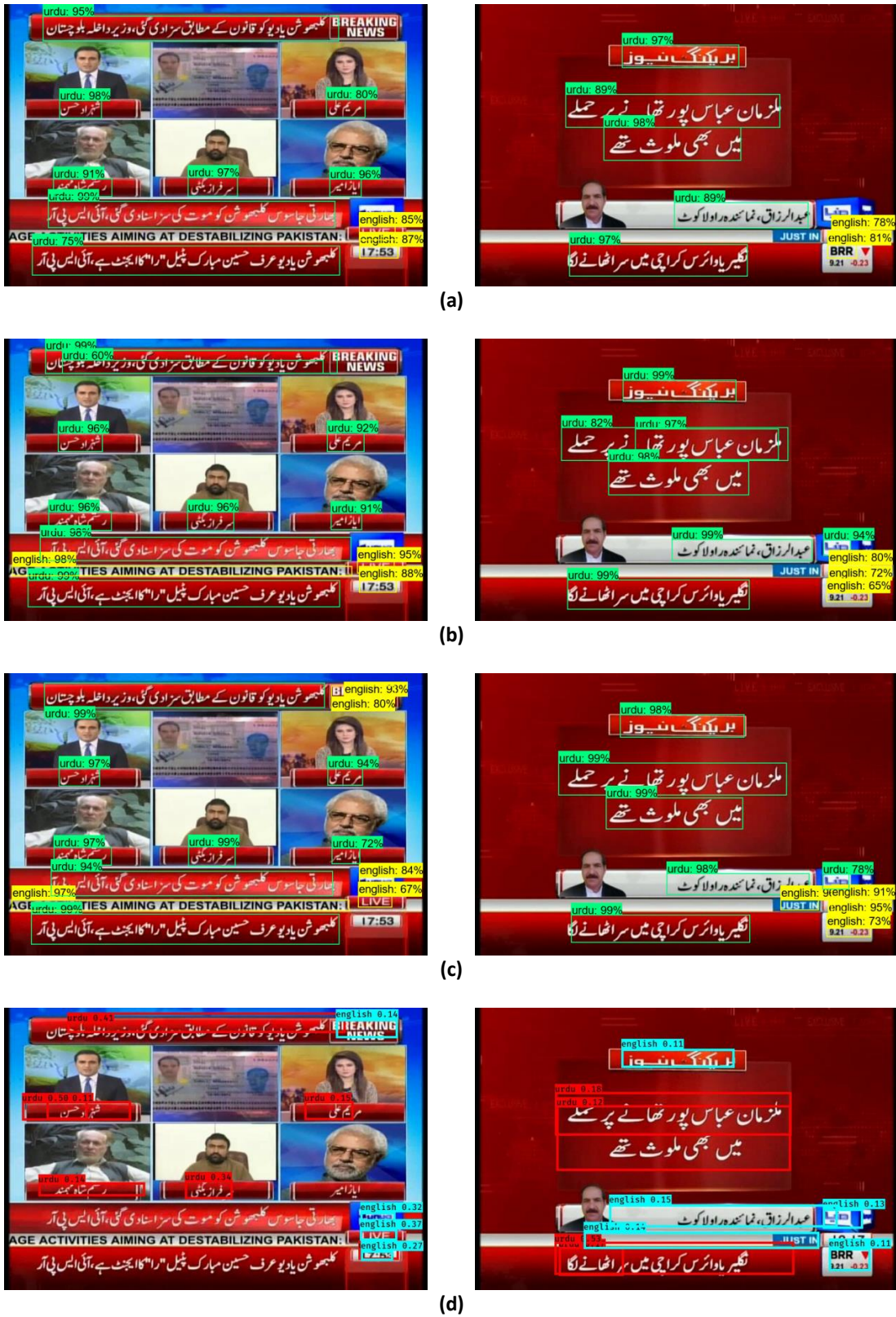
Figure 4.18: Detection output of hybrid text detection and script identification for different detectors (a): SSD (b): R-FCN (c): Faster RCNN (d): Yolo
