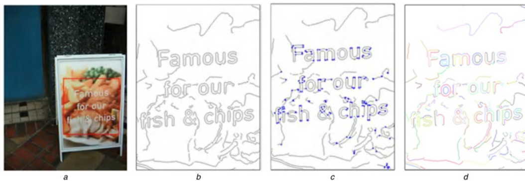
Figure 2.6: Edge segmentation example (Image Source [84]) (a): Original image (b): Edge image, (c): Segmentation points (d): Edge segmentation with different colors
