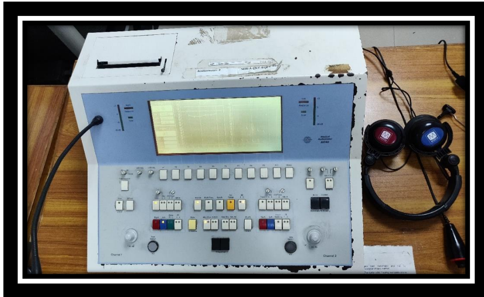
Figure 3.12 Pure Tone Audiometer for recording hearing thresholds (dB)
