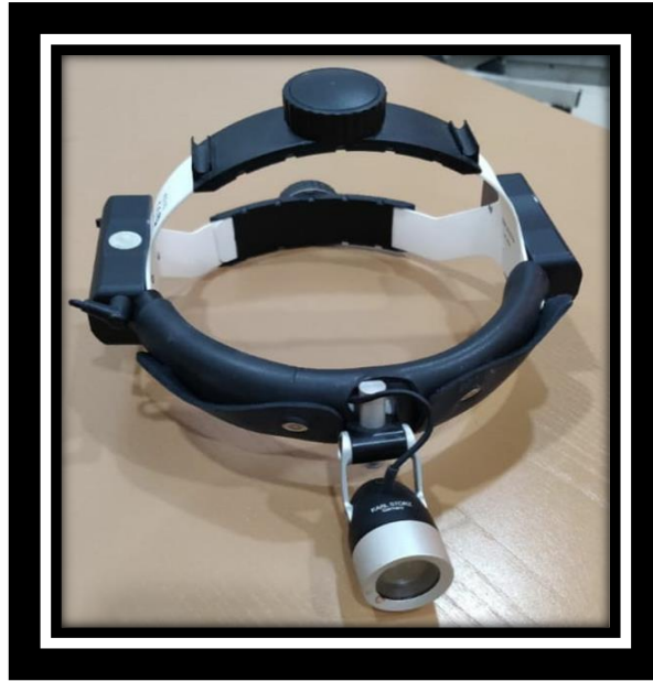
Figure 3.9 Head light used to focus light into cavity under inspection
