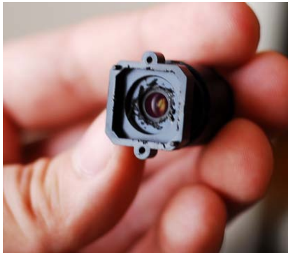
Figure 3.5 IR filter Removed
