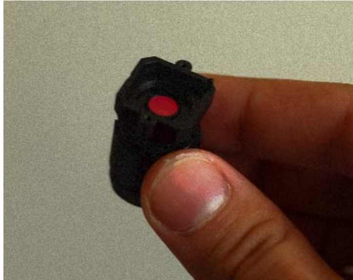
Figure 3.4 IR sensor inside PS3 Eye cam
