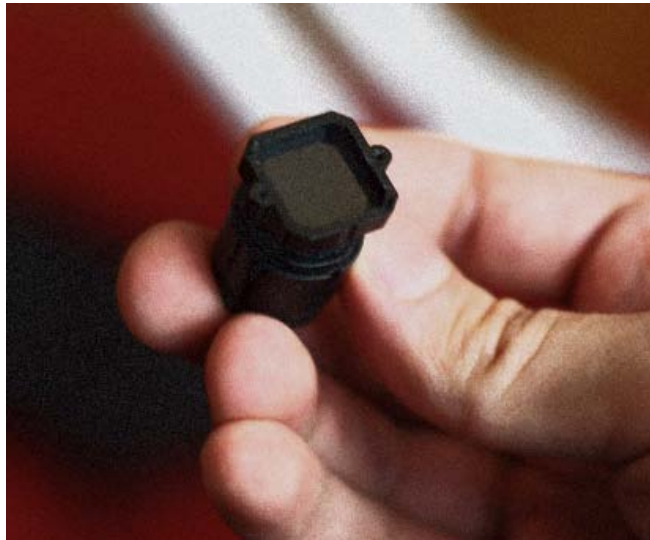
Figure 3.6 IR Filter Installed
