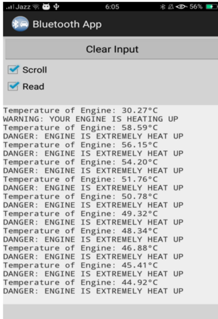
Figure 8.13: Transmitting Bluetooth Module Data
